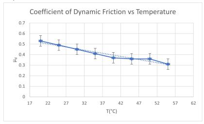
Graph 1 shows the relationship between the experimental values of Temperature and and the calculated coefficient of dynamic friction. According to the graph, the dynamic coefficient of friction between the surfaces is affected by the Temperature of the lubricant and this relationship is linear. As the temperature of the engine oil increases the dynamic coefficient of friction decreases.
